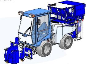
The triple headed grinding machine is being used for grinding of large asphalt or concrete surfaces.
