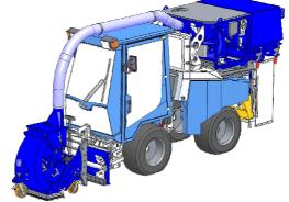
The removable scarifying head is been used for removing layers from asphalt, concrete or road marking stripes.
